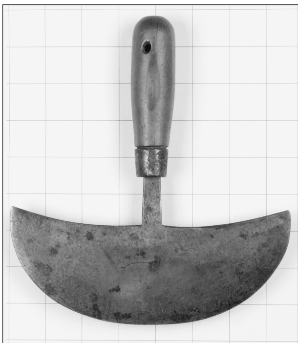
Figure 2. Eighteenth century, blacksmith-made, single-blade chopping knife. (Scale: 2.5 cm grid) (Photo by author; Museum of American Heritage)
